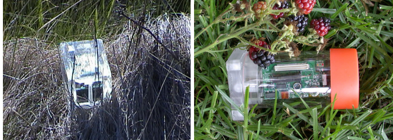
Figure 18.3. Acrylic enclosures used at different outdoor applications.
